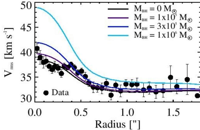
FIG. 12.— 1-D  $V_{\text{rms}}$  vs. JAM prediction of BH mass models. All models are fixed to the best-fit anisotropy parameter ( $\beta_z = 0.05$ ), mass scaling factor ( $\gamma = 0.890$ ), and inclination angle ( $i = 20^\circ$ ). The data are binned radially. The models show the JAM model predictions at a range of BH masses; the data clearly favors a low BH mass  $\lesssim 10^5 M_\odot$ .
