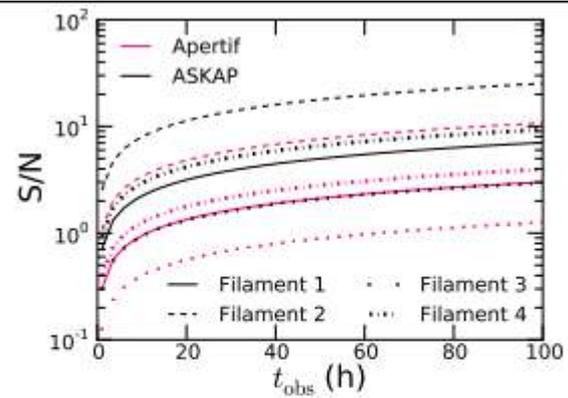
**Figure 10.** Expected signal to noise of the simulated filaments with the HI survey instruments Apertif and ASKAP. We assume an angular resolution of 10 arcmin and a frequency bandwidth of 0.6 MHz. The color of the lines denotes the instrument and the linestyle shows for which filament it is.
